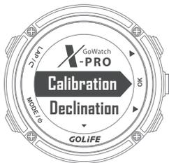
[ Calibration ] : For initiating or re-calibrating the Compass, press [ OK ] and place the watch on a horizontal surface with its face down. Turn the watch at the spot until the message of successful calibration shows up.
