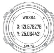
On completion of positioning, coordinates of current location WGS84 is displayed.
