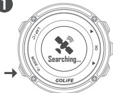
Press [ MODE ] and wait for GPS search and positioning ( Press [ OK ] twice to skip GPS search for Indoor Cycling and Indoor Running ).
