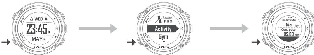
※ In Daily Mode, press [ OK ] Key to switch-over among Clock Screen, 3-Sensor Screen ( Atmosphere/ Altitude/ Temperature ), Compass, Daily Track Screen, etc. ( Press [ UP ] or [ Down ] in each screen to switch among different data fields. )
