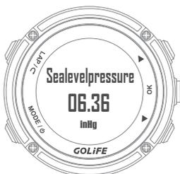
[ By Current Elevation ]: For example, after entering current altitude when you reach an altitude benchmark in the mountain, GoWatch will automatically calibrate the atmosphere value.
